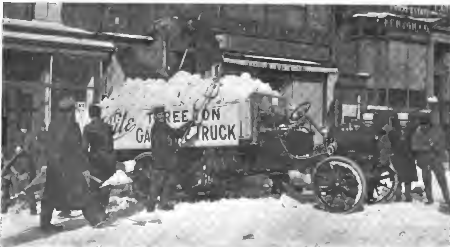
White Three-Ton Gasoline Truck Removing Snow in New York City
